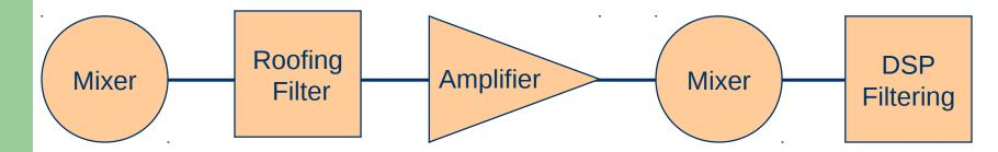
On CW, the wider the roofing filter, the worse the problem. The more signals inside the roofing filter, the more the DSP filtering is stressed. Example: The IC-7600 has a roofing filter that is about 1/3<sup>rd</sup> the width of the Pro III, and a stronger front end.
